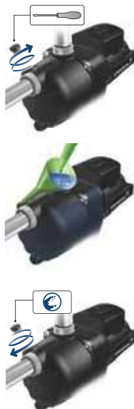
Fig. 8 Priming the pump
