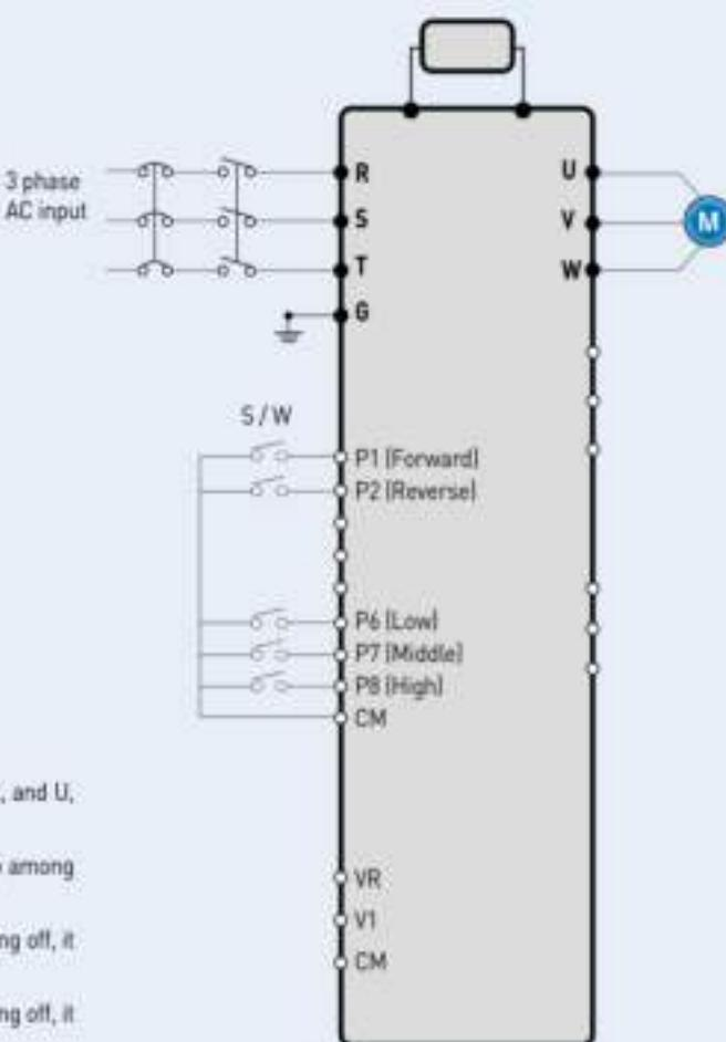
1. Please make sure that R, S, T are connected to 3 phase AC input, and U, V, W are also motor connection terminals.
