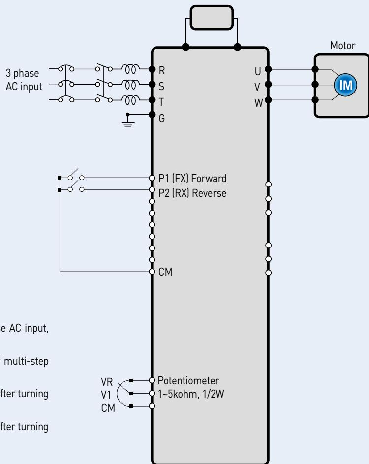
1. Please make sure that R, S, T are connected to 3 phase AC input, and U, V, W are also motor connection terminals.
